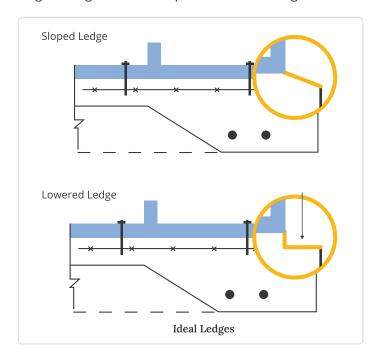
The person who builds the frame for pouring your slab can form a sloped or lowered ledge by placing six-inch boards inside the form boards, ¾" of an inch lower than where the top of the slab will be. If you decide to leave the ledges at the same level as the rest of the slab, you should apply a concrete sealant around the base rail of your garage after it is installed to prevent water from seeping into the garage.
